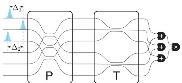
Figure 2: Decomposition of interference network and setup for the detectors.
