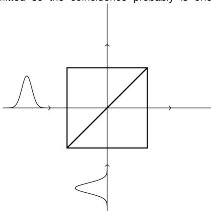
Figure 1: Two-photon interference at a beam-splitter
